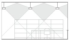
Suspended light structure with integral, direct-indirect luminaires for fluorescent lamps, and integral downlights for lowvoltage halogen lamps.
